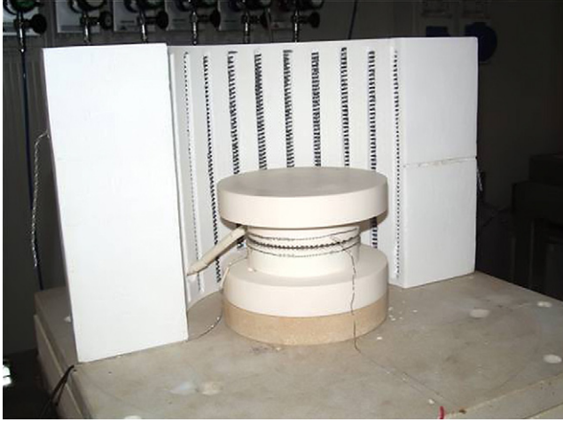
Fig. 5. Detail of the single fuel cell test rig in the fuel cell laboratory at the University of Perugia.
